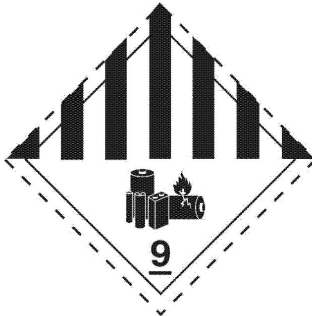
(b) In addition to complying with § 172.407, the background on the LITHIUM BATTERY label must be white with seven black vertical stripes on the top half. The black vertical stripes must be spaced, so that, visually, they appear equal in width to the six white spaces between them. The lower half of the label must be white with the symbol (battery group, one broken and emitting flame) and class number “9” underlined and centered at the bottom in black.
