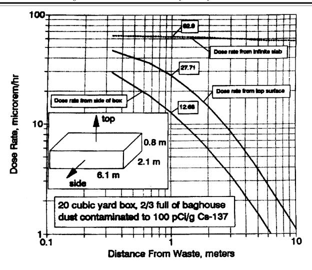
Figure 1. Shape Factor Plot for 20 Cubic Yard Container
