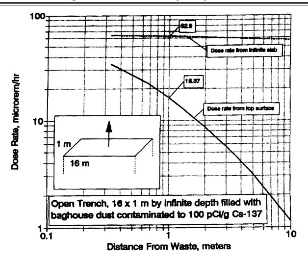
Figure 4. Shape Factor Plot for Reference Open Trench
