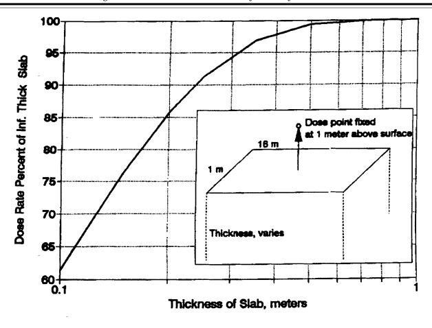
Figure 7. Dose Rate (Expressed as a Percentage of an Infinite Slab Dose Rate) as a Function of Trench Thickness
