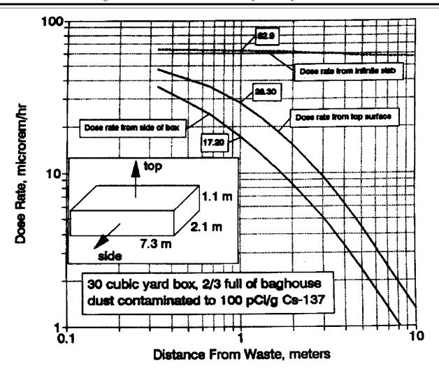
Figure 2. Shape Factor Plot for 30 Cubic Yard Container
