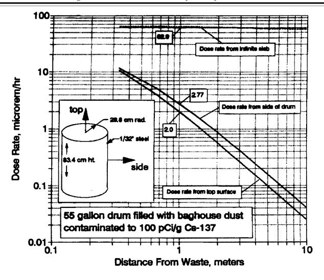
Figure 5. Shape Factor Plot for Standard 55 Gal. Drum
