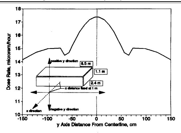
Figure 8. Dose Rates as a Function of Vertical Distance
