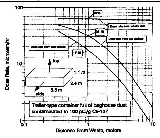
Figure 3. Shape Factor Plot for Trailer-Type Container
