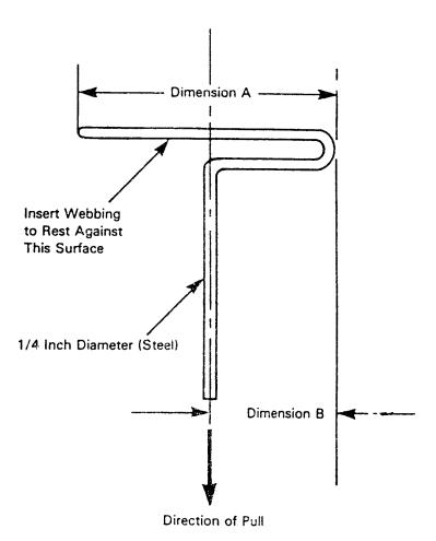
Dimension A - Width of Webbing Plus 1/2 Inch Dimension B - 1/2 of Dimension A
