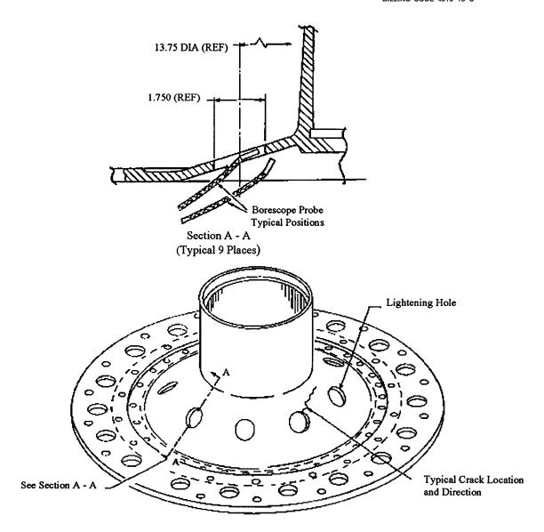
Borescope Inspection of Second Stage Lower Planetary Plate Figure 2
