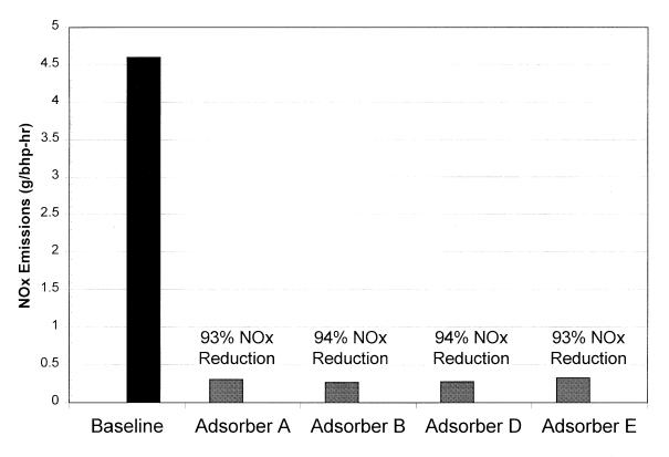
Figure III-1. NVFEL NOx Adsorber SET Composite Results
