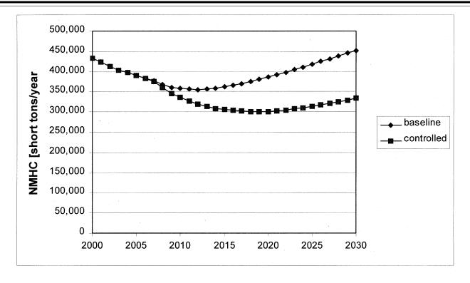
Figure II.D-3: Projected Nationwide Heavy-Duty Vehicle NMHC Emissions
