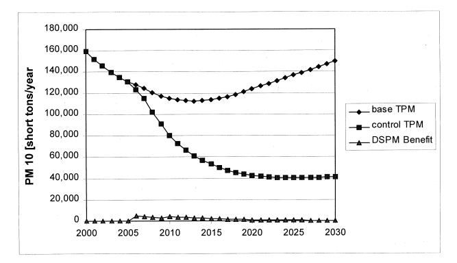
Figure II.D-2: Projected Nationwide Heavy-Duty Vehicle PM Emissions
