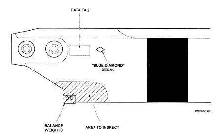
Figure 1. Tail rotor blade inspection.
