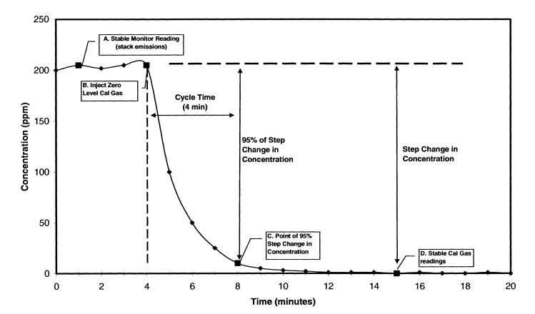
Figure 6b. Downscale Cycle Time Test
