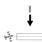
ADVANCE TO PERMIT CENTER LINE TO BE FLOWN WITH ONLY MINOR COORDINATED CORRECTIONS AIRCRAFT WILL BE FLOWN DOWN AN EXTENSION CORRECTION ESABLISHED SUFFICIENTLY IN OF THE RUNWAY CENTER LINE WITH DRIFT
