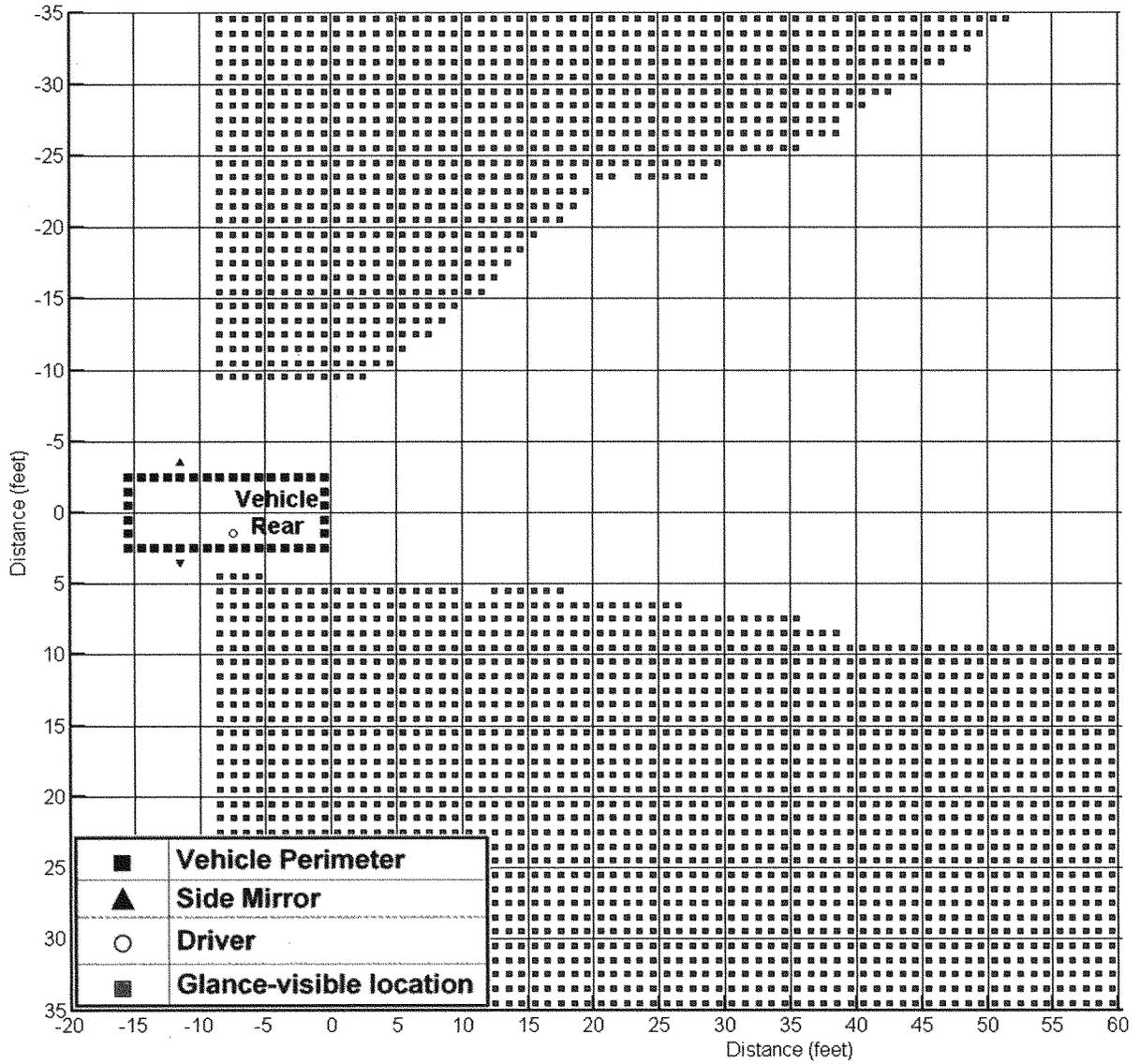
Figure 7. Direct Field of View Measured Using a 50<sup>th</sup> Percentile Male Driver: SUV (2007 Jeep Commander 4x4).
