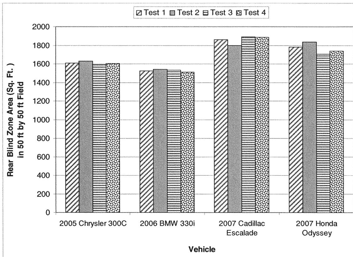
Figure 13. Rear Blind Zone Area Measurement Repeatability Results
