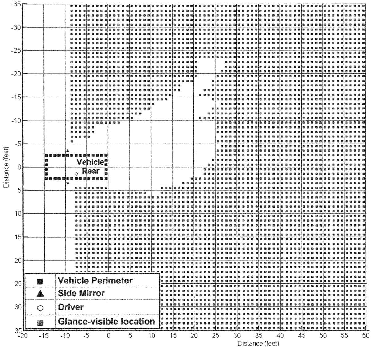
Figure 5. Direct Field of View Measured Using a 50<sup>th</sup> Percentile Male Driver: Passenger Car (2007 Chevrolet Cobalt, Coupe).
