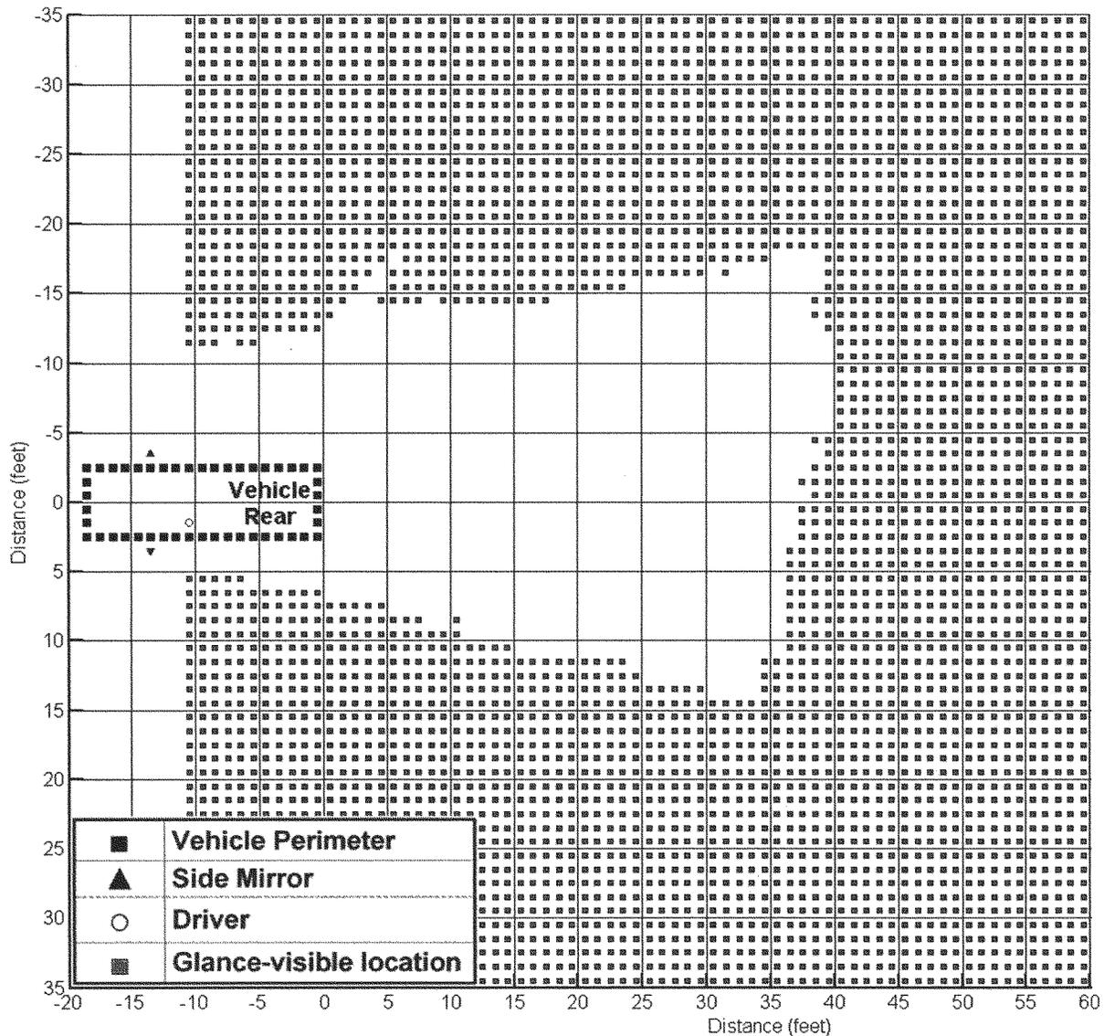
**Figure 8. Direct Field of View Measured Using a 50<sup>th</sup> Percentile Male Driver: Pickup Truck (2006 Ford F-150, 4x4, 4-door Extended Cab).**
