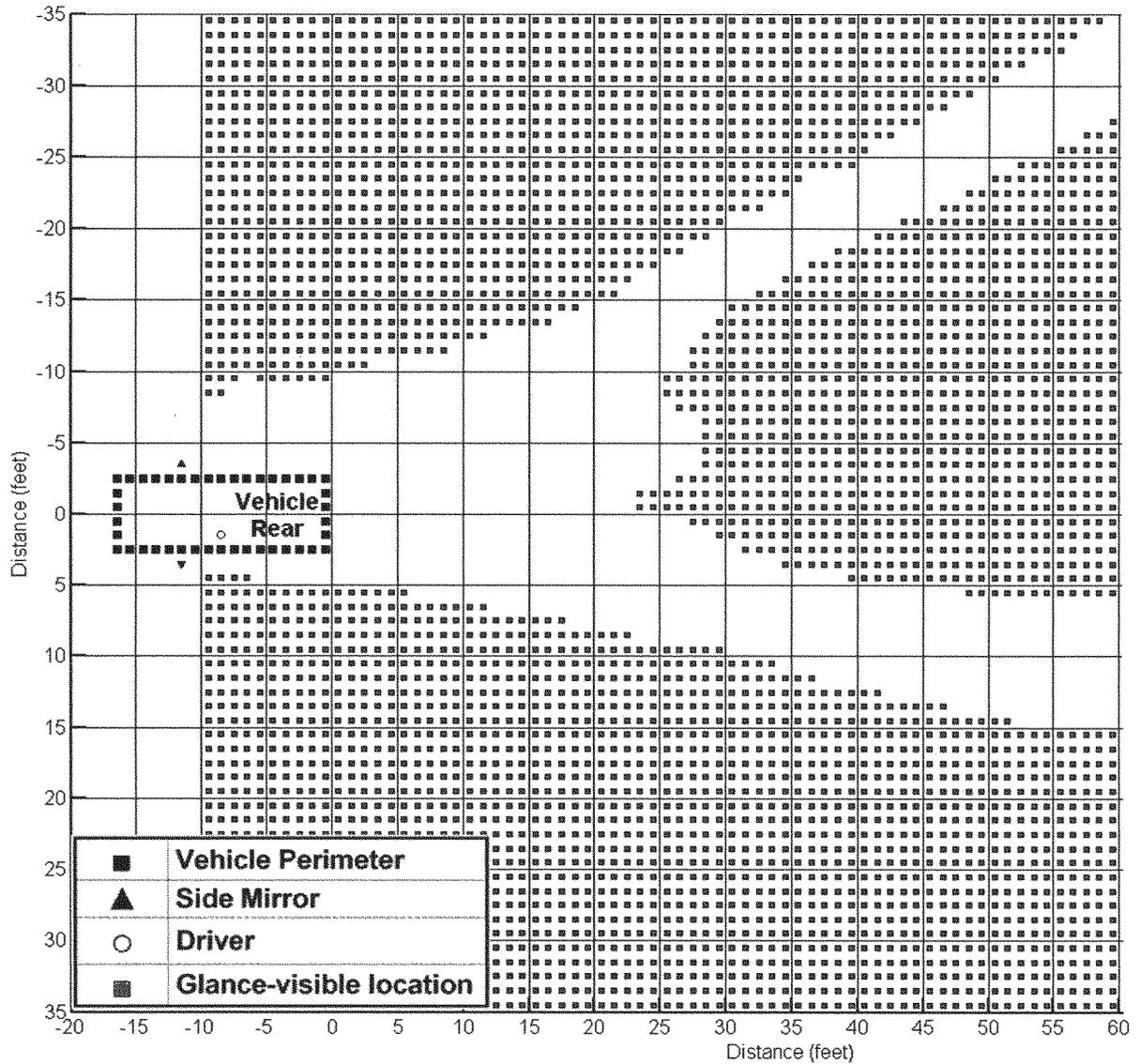
Figure 6. Direct Field of View Measured Using a 50<sup>th</sup> Percentile Male Driver: Minivan (2007 Honda Odyssey).
