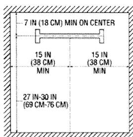
Figure 13 -- Clearances for Fixed Ladders in Wells
