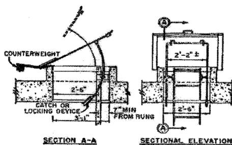
Figure D-3 -- Counterbalanced Hatch Cover at Roof
