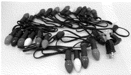
Picture 2: Parallel-connected screw-base bulbs light string
