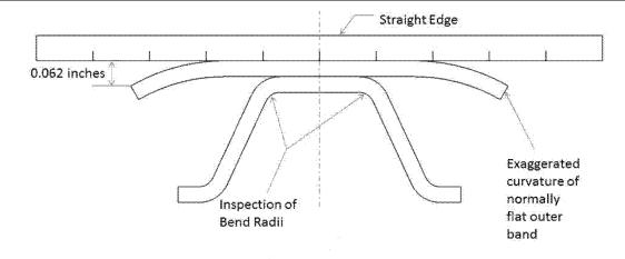
Figure 1 to paragraphs (h)(1)(iii) and (v) of this AD: Cross section of v-band
